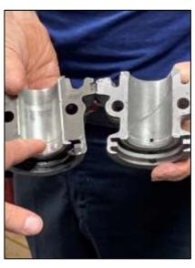
We wanted to check the oil gap and found out there was no engine bearing shims (this engine was a rebuilt unit but not correctly). We had .002 clearance (which is too much). After working on the cap we were able to reduce that to approximately .0013. Should be between .001 and .0015.
